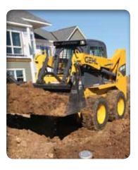
**ACCELERATE RAPIDLY with** maintenance-free, radial-piston drive motors with high start-up torque and maximum ground speeds up to 13.9 mph<sup>1</sup> (22.4 km/hr).
