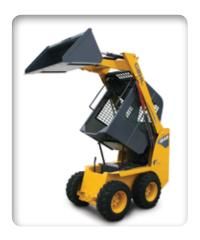
service made easy with a large engine cover and tilt-back ROPS/FOPS that allows access to daily maintenance points, as well as service access when needed.
