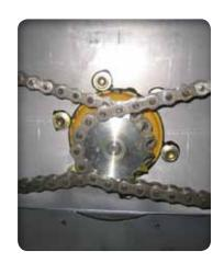
**HEAVY-DUTY DRIVETRAIN** is composed of durable components. Adjustments can be made to the simple "bow-tie" chain system from outside the unit.
