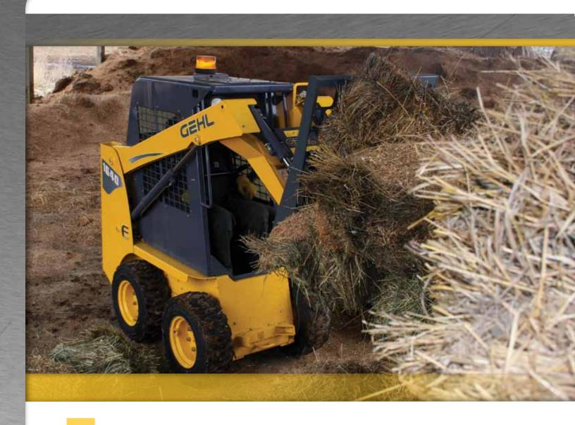
Super-compact and tough, the 1640E skid loader from Gehl can go where other machines can't. A width as narrow as three feet makes maneuvering through narrow doors and alleyways easy, while a strong 850-pound (386 kg) rated operating capacity makes a huge dent in the workload.
