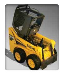
SERVICE IS A SNAP with a swing-open rear door, flip-up engine cover, and tiltable ROPS/FOPS that fully exposes maintenance points at the engine, battery, and filler caps.
