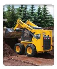
**HIGH OPERATING CAPACITIES** from 1,650 lbs. (748 kg) on the 4640E Power2 to 2,900 lbs. (1315 kg) on the 6640E with the optional counterweight.
